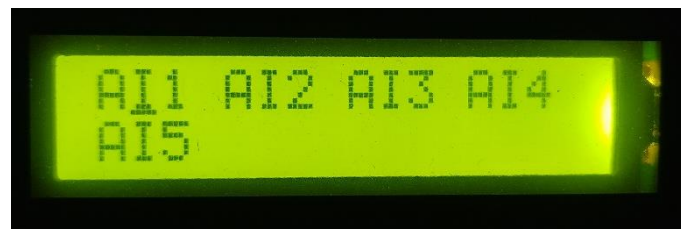
Fig. 22 shows Threshold channel selection screen
