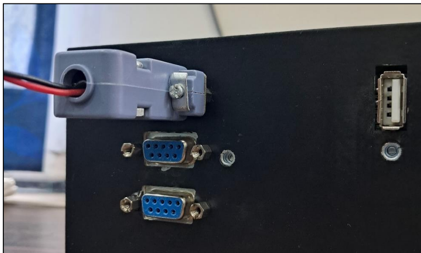
Fig 34. Shows RS485 connection to DSmart400 Device
