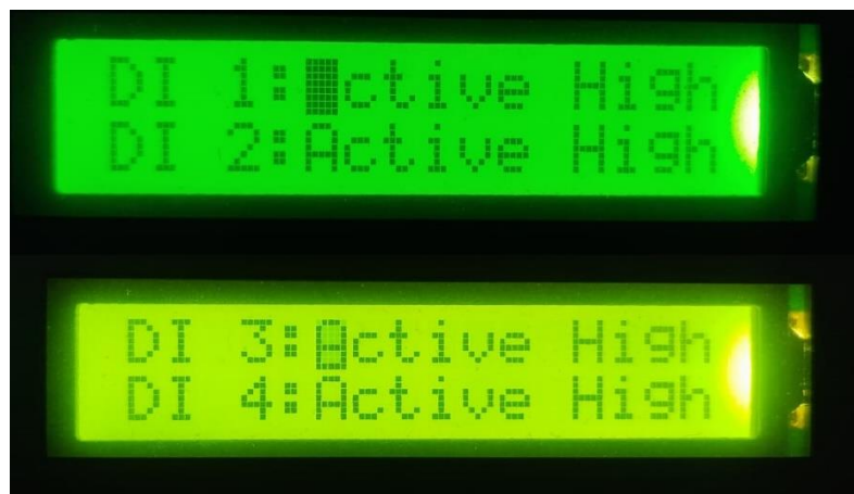
Fig 21. Shows Digital input active High/Low Option
