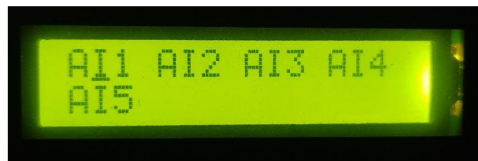
Fig 11. shows cursor on 'I', AI2 Channel is selected. Press 'ENTER' to enter it
