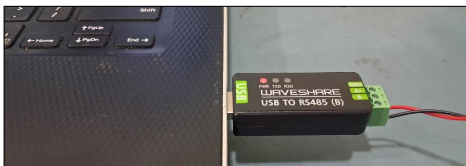
Fig 33. Shows Rs485 connection with computer
